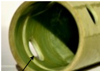
Machining of an internal groove and laying of a stainless-steel ring
